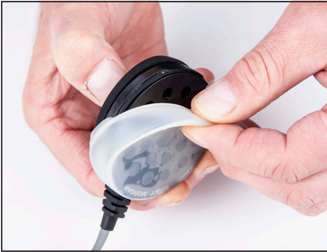
Removing the rubber cover from the earphone.
