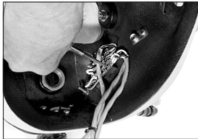
The terminal block is where you will disconnect the earphones from the helmet or mask.
