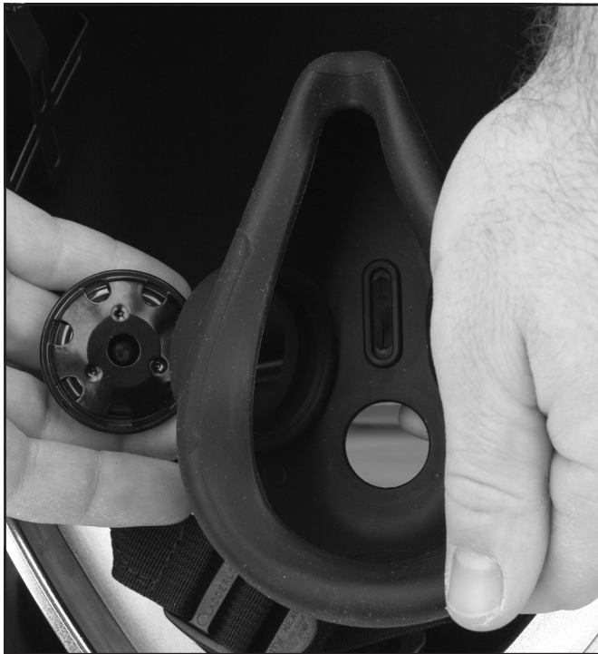
Install the microphone into the oral nasal mask.
