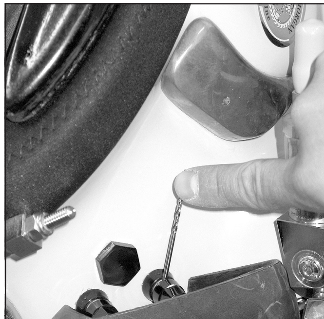
Make sure the holes in the binding posts are properly aligned so that you will be able to thread the communications wire through them easily when you are ready to dive.
