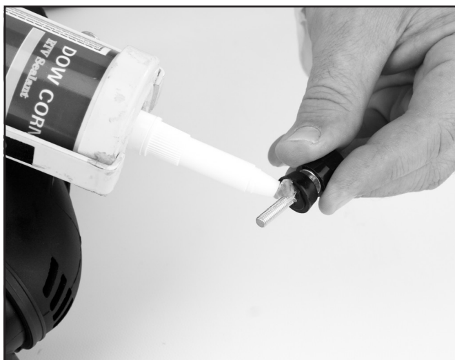
The communications posts are sealed in place with silicone sealant.
