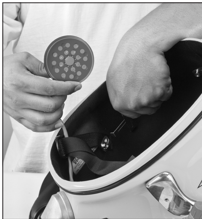
Remove the earphones from the retainers to inspect the speaker cones.
