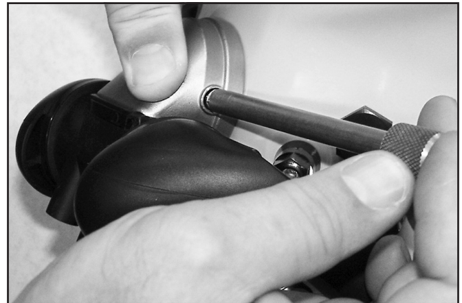
The water dump adapter cover must be properly fastened to the helmet water dump.
