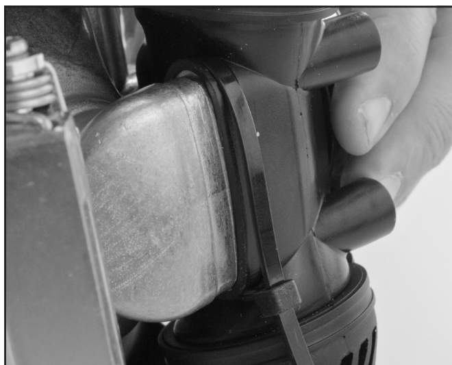
These two must align before tightening the tie wrap. Insert the regulator into the pod.
