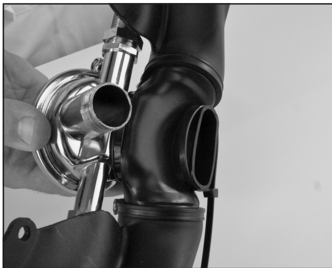
Pre-install the tie wrap.
