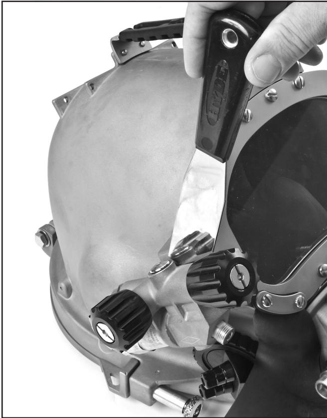
A thin putty knife can be pushed between the side block and the helmet shell to help remove the side block.
