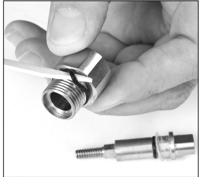
Use a toothpick, credit card, or other non-metal objects to remove the O-rings for cleaning and replacement. Note that the bonnet on the EGS valve is shorter than the bonnet on the defogger valve.
