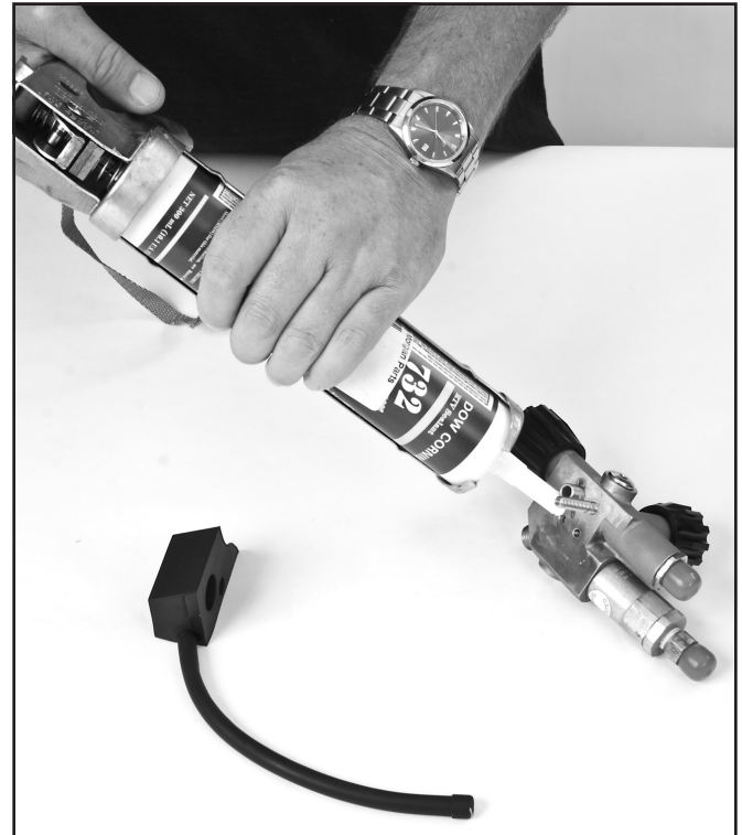
A small amount of silicone sealant must be evenly applied to the side block prior to installation on the helmet shell. Use only Dow Corning® RTV 732 Multi Purpose sealant or equivalent.
