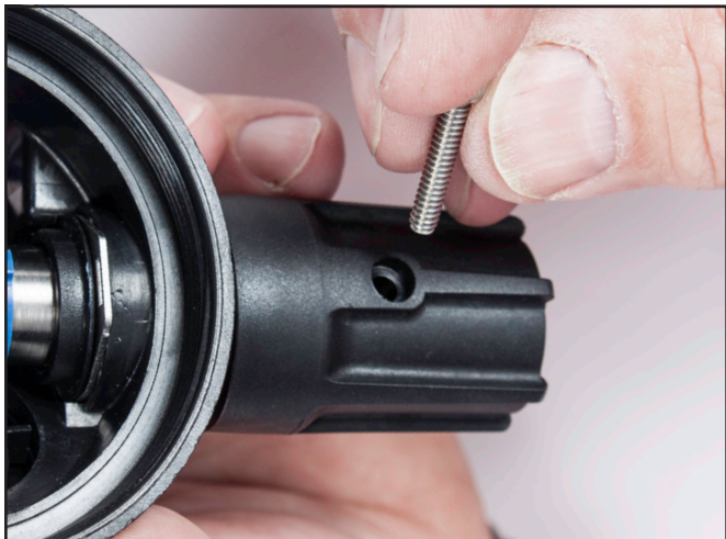
Install the knob screw using the \frac{7}{64} inch hex wrench.
