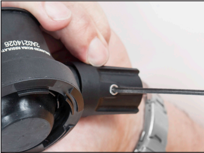
Remove the adjustment knob screw.
