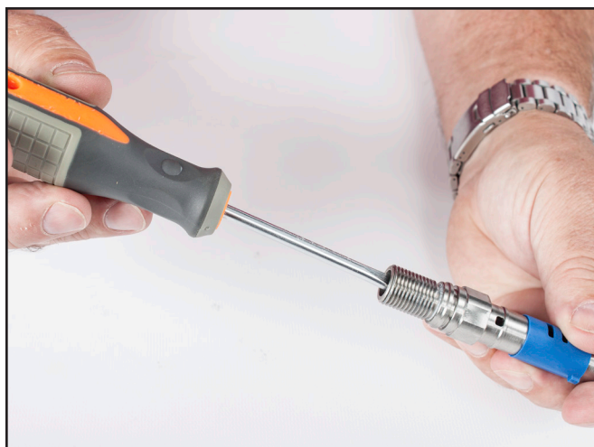
Using a medium flat blade screwdriver, thread in about three full turns.
