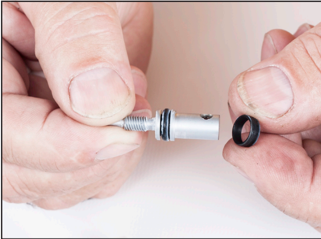
Separate the spacer.
