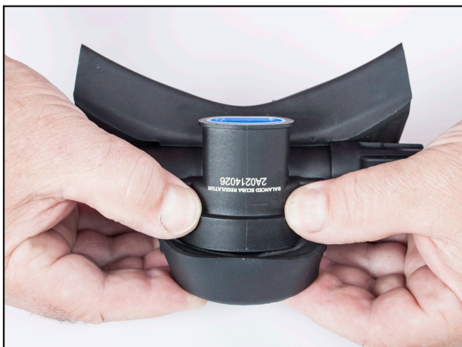
Continue pushing the cover onto the regulator.
