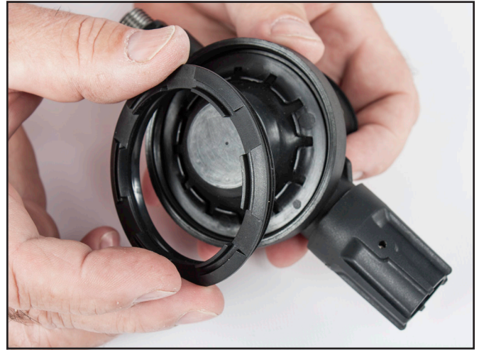
Install diaphragm retainer ring.
