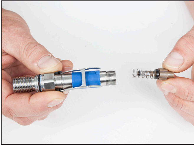
Remove the balance spacer, spring and washer.
