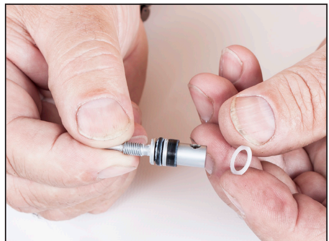
Separate the thrust washer.
