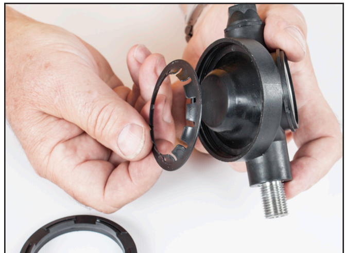
Remove the surge dam.
