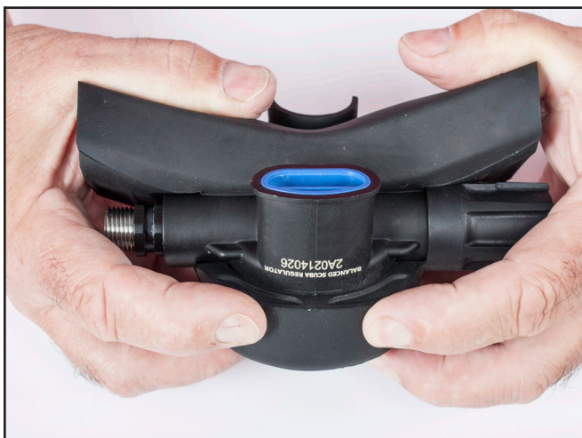
Stretch the upper portion of the regulator shroud/exhaust cover over the top of the regulator and make certain all areas between the two are aligned and mating. Correct alignment/position of the cover and regulator.
