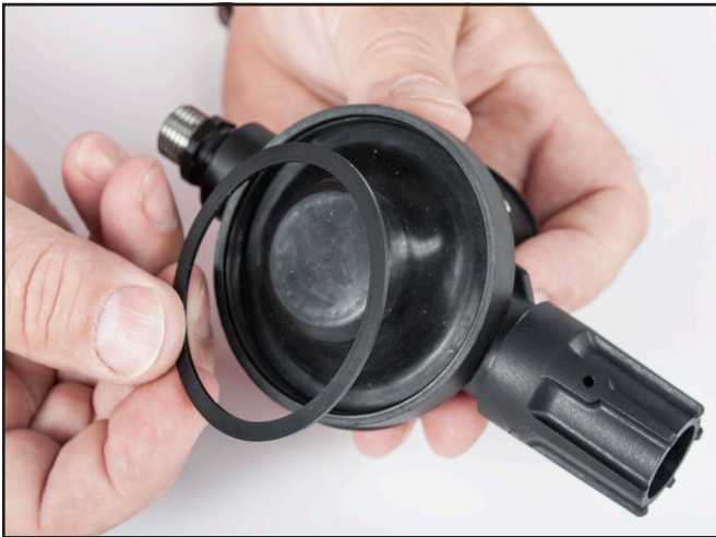
Install the diaphragm washer.
