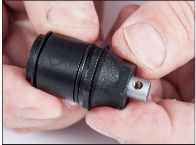
Hand tighten the end cap packing nut as much as possible.
