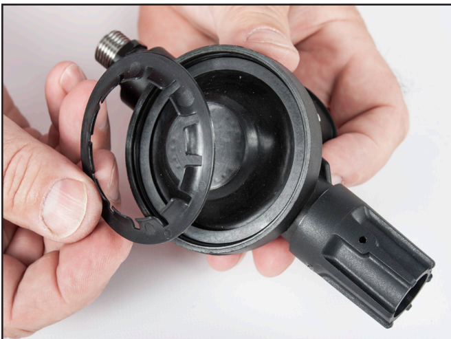
Install diaphragm surge dam.
