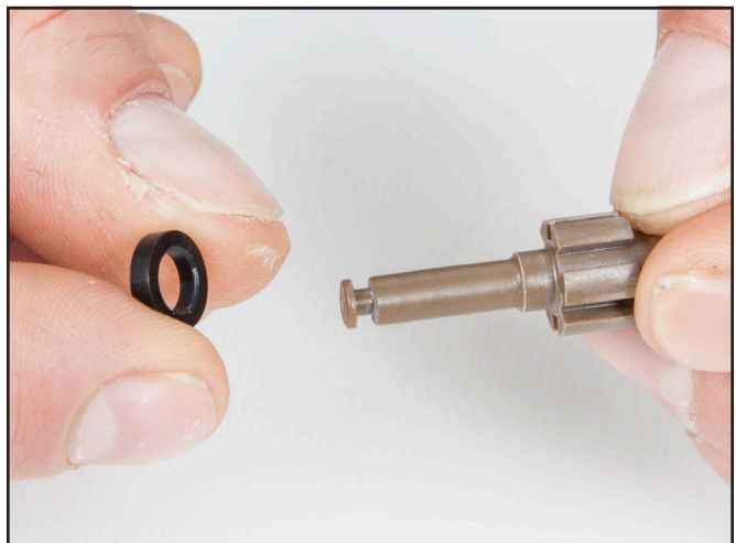
Install the washer onto the balance spacer
