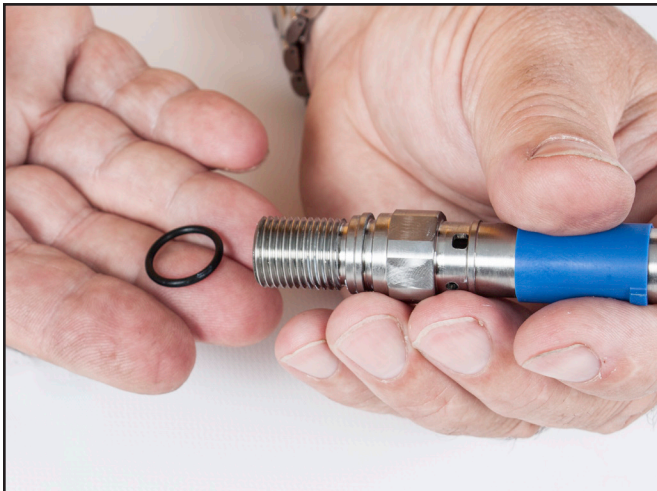
Remove the O-ring from the main tube.
