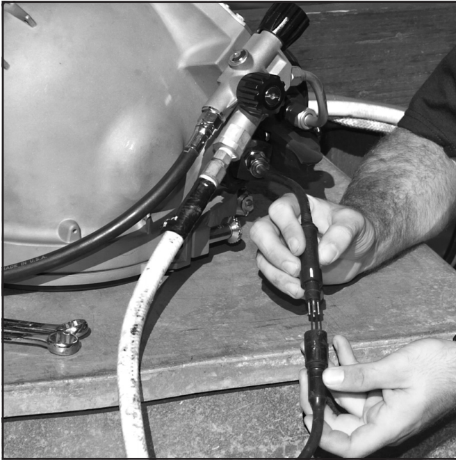
Connecting the waterproof connectors.
