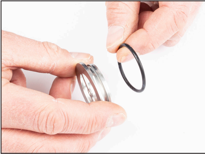
13) Remove Housing Retainer Ring.
