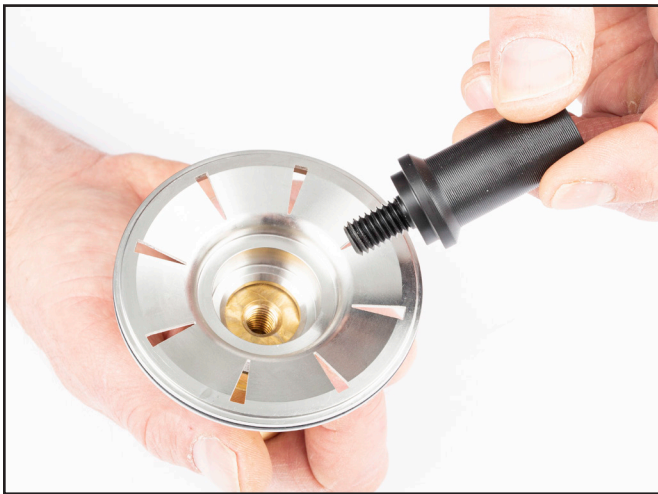
7) Unthread handle and remove tools from Valve Seat.
