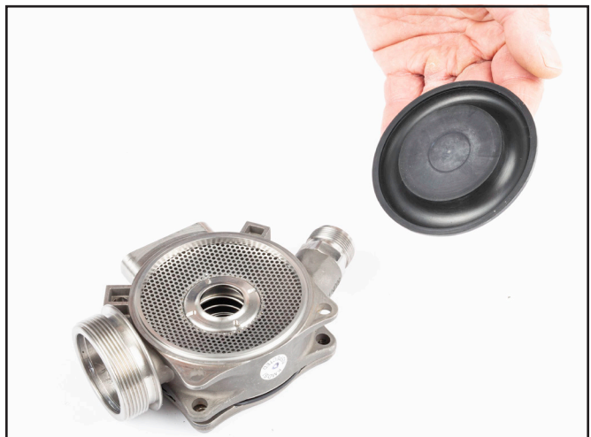
19) Complete disassembly of exhaust regulator—Bottom cover, 2nd Stage Diaphragm and Spring.
