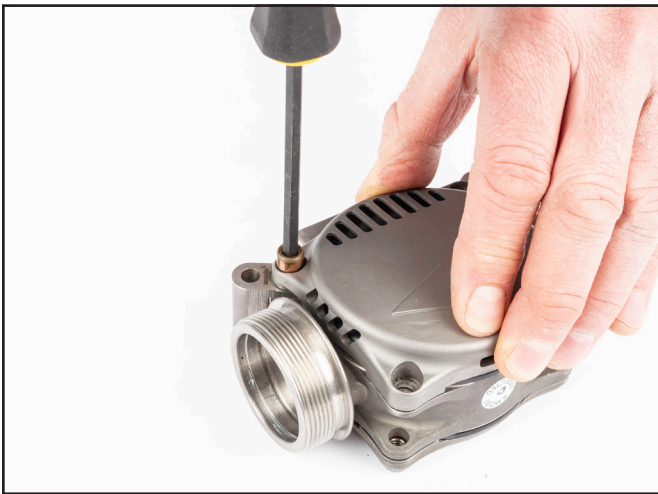
17) Remove Mount Blocks. Note arrow direction for future reinstall.
