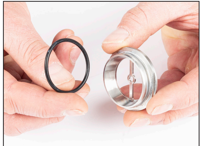
7) Insert the puck seal with O-ring evenly into the exhaust valve body, and push in EVENLY until completely seated.
