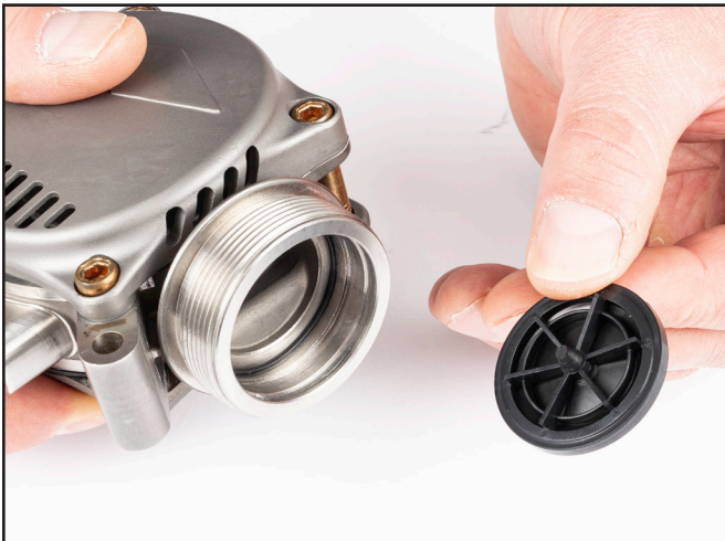
5) Insert Retainer Ring into OPRV body.
