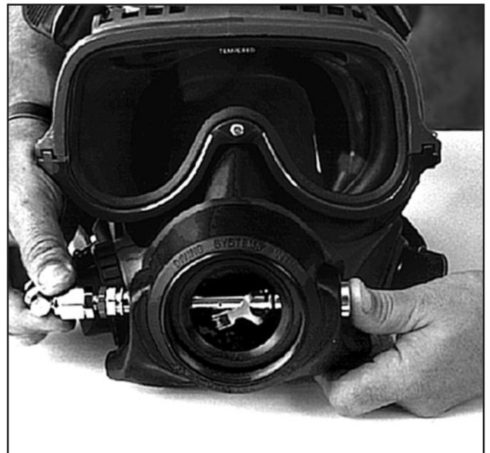
Push the main tube out enough to allow the lever arm to be removed.
