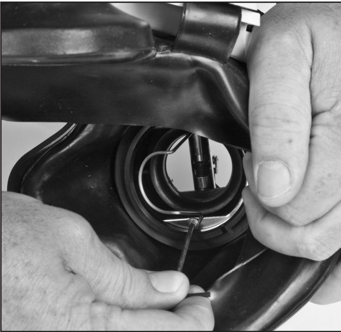
Tighten the screws for the nose block wire retainer.
