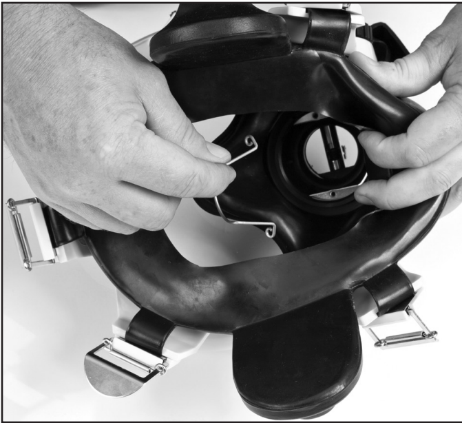
After the regulator is adjusted, install the wire retainer for the equalizing device.
