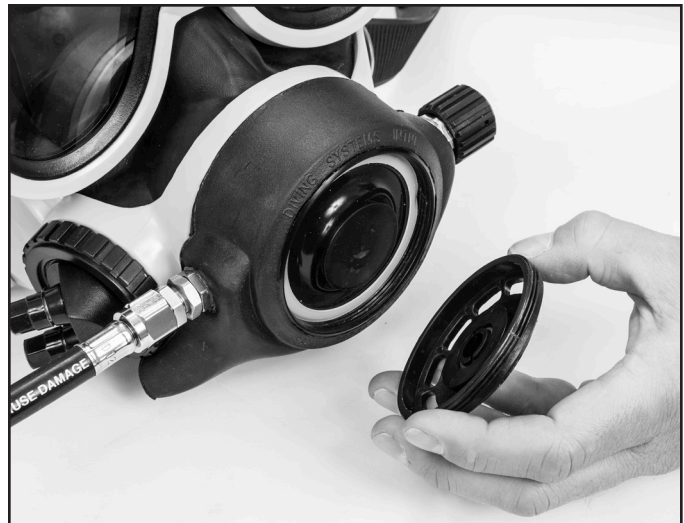
Remove the regulator cover.
