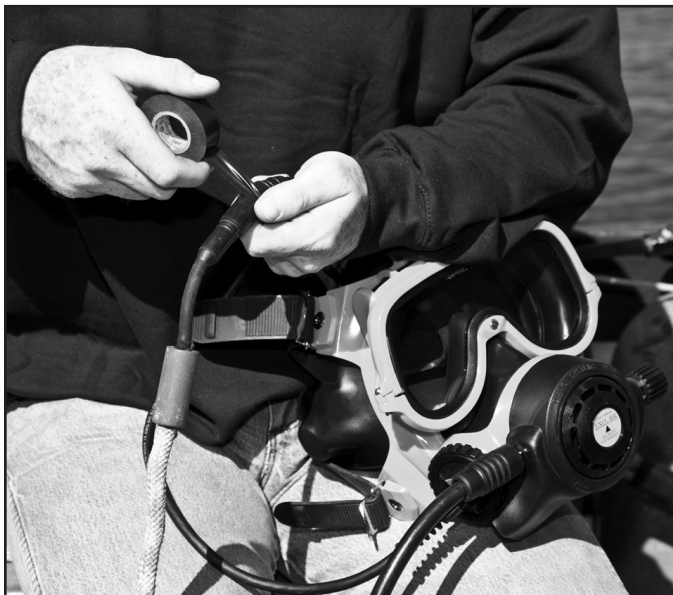
You can use electrical tape to secure the waterproof connectors together.
