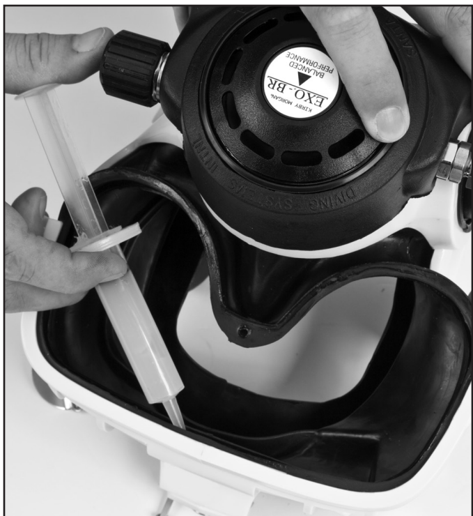
Apply silicone grease to the mask seal.
