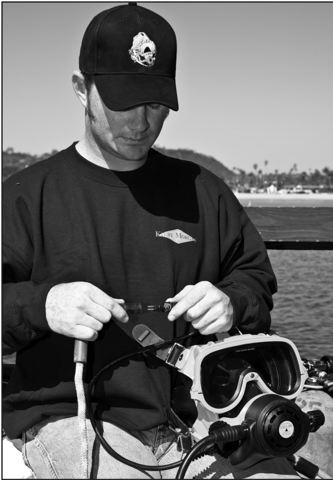
Connect the waterproof connectors without twisting them.
