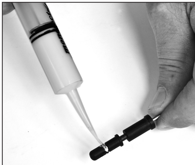
Be sure to lubricate the inlet valve sparingly with silicone grease.
