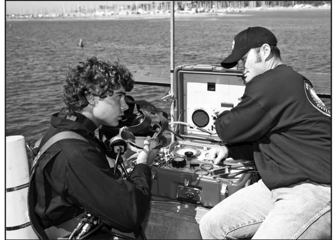
Always test the communications before the diver gets in the water.
