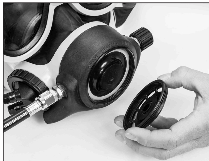
Install the regulator cover.
