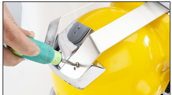
Reinstall the two top weight screws and washers
