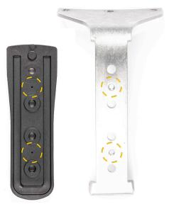
Underside of the handle top indicating where to drill holes (#7, 0.201") and corresponding holes on the topside of the handle, in order to use the original grip mounting holes in the handle (10-32 UNF Screw). There are two options for creating holes that can be used for mounting light and camera brackets to the handle:
