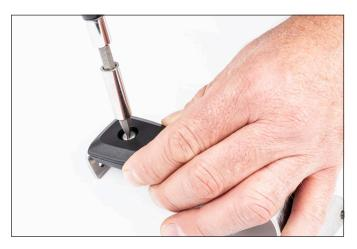
8) Apply Loctite<sup>®</sup> 248 to the screws and install. Torque to 15 Inch Pounds (1.7 Newton Meters).
