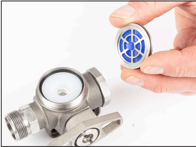
2) Remove O-ring from valve seat.
