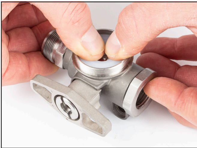
4) Lubricate and install O-ring on top of Exhaust Port Seal.
