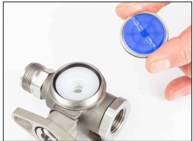
8) Ensure Valve is opening away from body.
