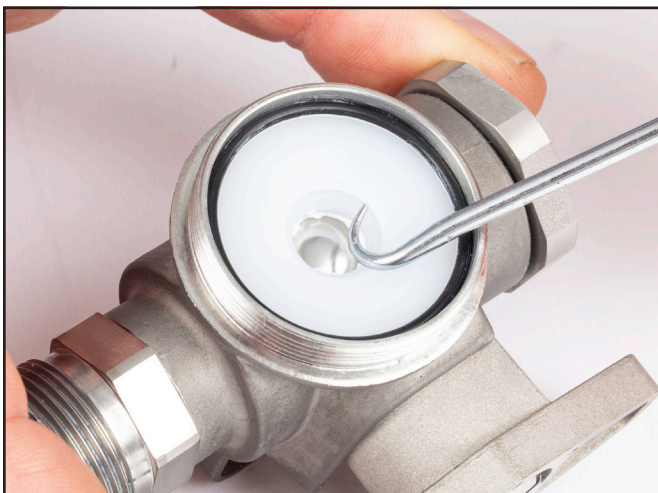
3) Place tip of a hooked pick into groove found on leading edge of Exhaust Port Seal.
