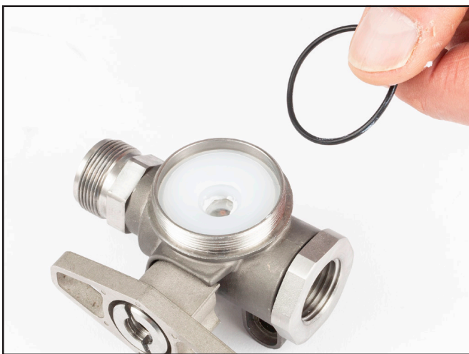
5) Install Butterfly Valve Seat onto correct side of seat.
