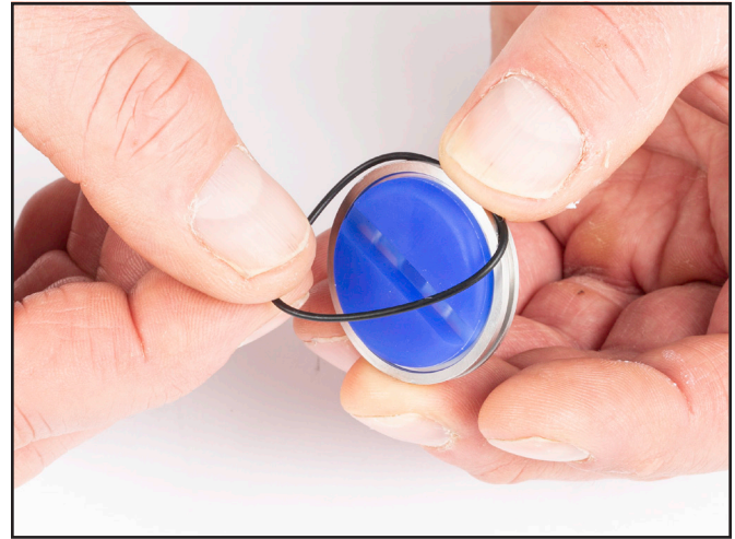
7) Place Butterfly Valve assembly on top of Exhaust Port Seal and O-ring.
